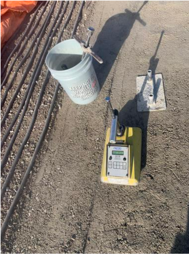
C2- Testing backfill lift at 100mm Arshdeep Grewal Feb 14, 2021 10:36 AM
