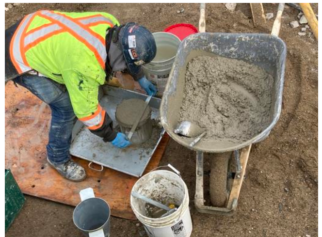
Testing for slump and air content
